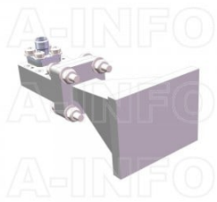
LB-42-15-C-KFSPO Standard Gain Horn Antenna 18-26.5GHz 15dB Gain 2.92mm Female
